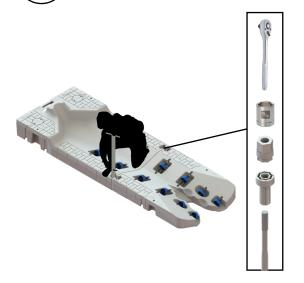
To install multiple Snap Ports align the two ports side-by-side. Use the two side pockets outlined to connect the ports by repeating steps 7-14 using CPLR-SET-GR.
